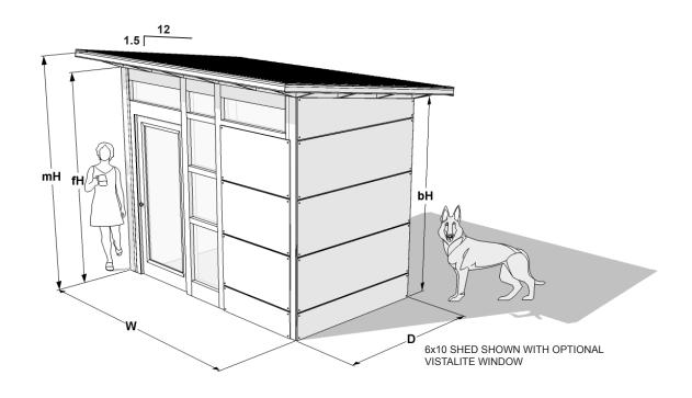
'W' = SHED WIDTH 'D' = SHED DEPTH 'mH' = MAX SHED HEIGHT 'fH' = FRONT WALL HEIGHT 'bH' = BACK WALL HEIGHT
