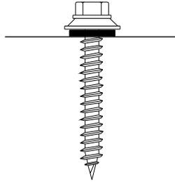
SEALING MATERIAL IS NOT VISIBLE; NOT ENOUGH COMPRESSION TO SEAL.
