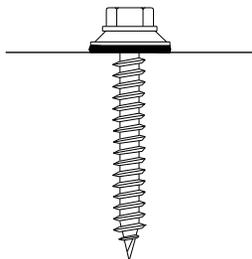
SEALING MATERIAL SLIGHTLY VISIBLE AT EDGE OF WASHER. ASSEMBLY IS WATER TIGHT.
