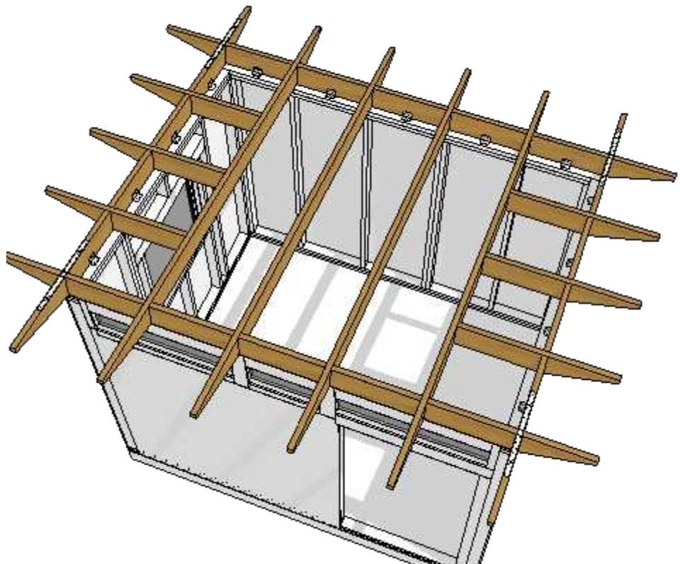
**INSTALL 6" RAFTER TIE SCREWS AT ALL LOCATIONS WHERE RAFTERS ARE PERPENDICULAR TO TOP PLATE:**
