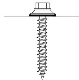
WASHER IS DEFORMED; SEALING MATERIAL PRESSED BEYOND FASTENER EDGE.
