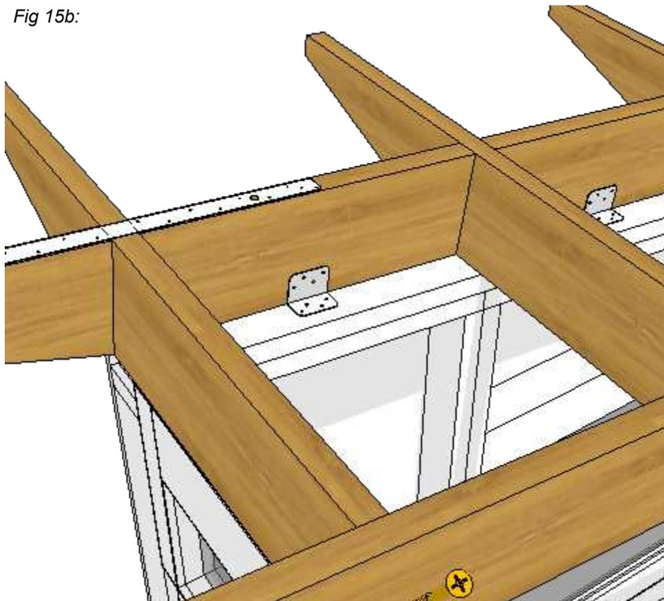
**INSTALL INTERMEDIATE RAFTER SECTIONS:**
