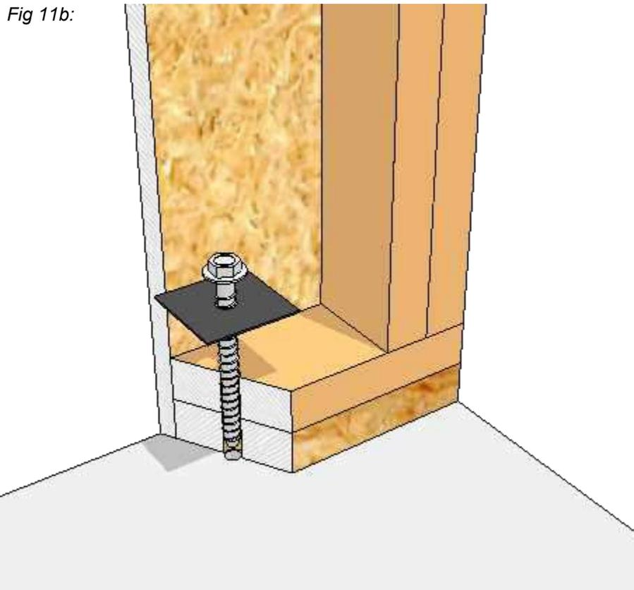
**INSTALL FINAL 3" SCREW AT ALL WALL PANEL CONNECTIONS:**
