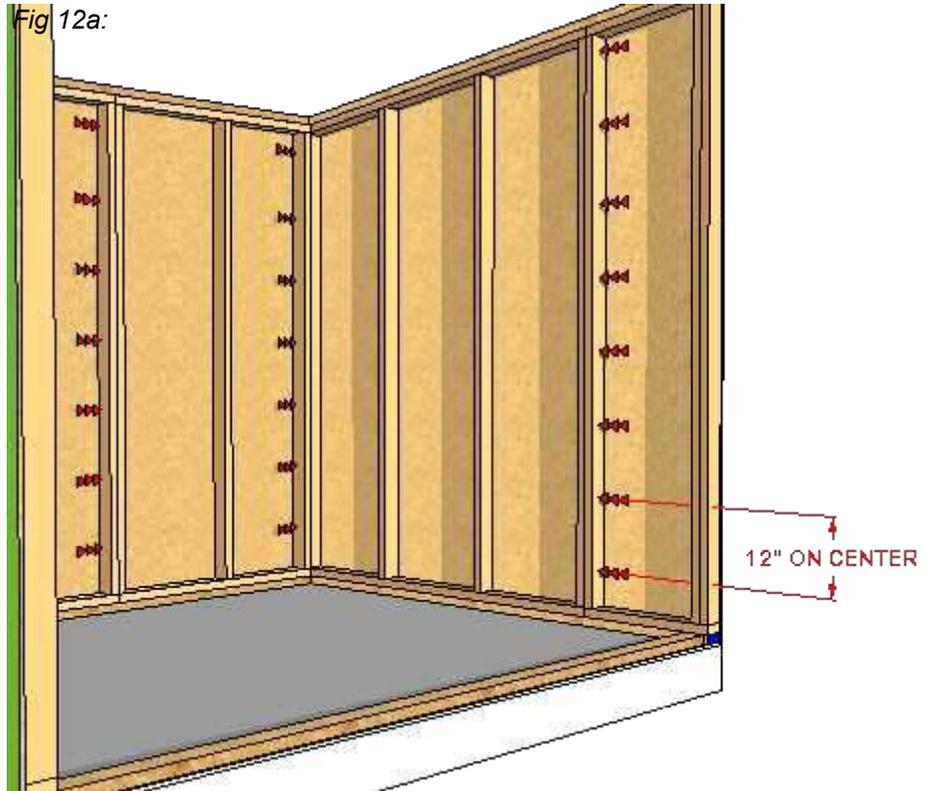
**NAIL WALL SHEATHING INTO TOP PLATE, SILL PLATE AND CORNERS:**
