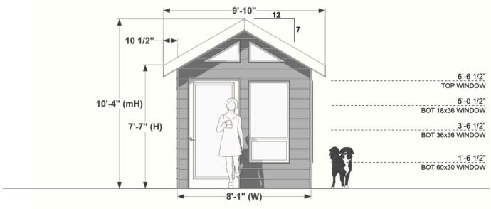
(D) = SHED DEPTH | (W) = SHED WIDTH | (mH) = MAX ROOF HEIGHT | (H) = SIDE WALL HEIGHT
