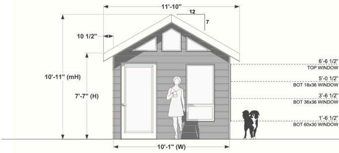
(D) = SHED DEPTH  $\mid$  (W) = SHED WIDTH  $\mid$  (mH) = MAX ROOF HEIGHT  $\mid$  (H) = SIDE WALL HEIGHT
