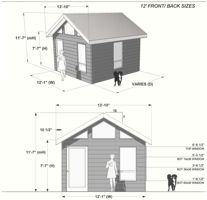
(D) = SHED DEPTH  $\mid$  (W) = SHED WIDTH  $\mid$  (mH) = MAX ROOF HEIGHT  $\mid$  (H) = SIDE WALL HEIGHT
