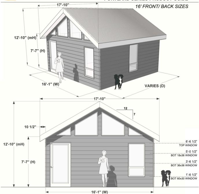
(D) = SHED DEPTH | (W) = SHED WIDTH | (mH) = MAX ROOF HEIGHT | (H) = SIDE WALL HEIGHT
