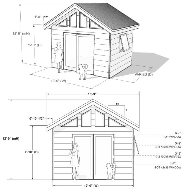
(D) = SHED DEPTH | (W) = SHED WIDTH | (mH) = MAX ROOF HEIGHT | (H) = SIDE WALL HEIGHT
