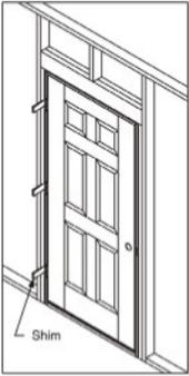
Leave door fastened and closed with transport clip.
