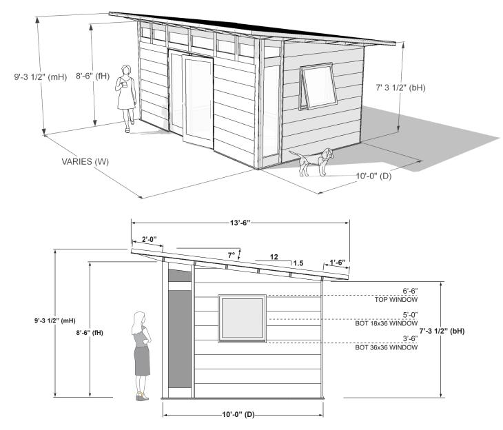
(D) = SHED DEPTH | (W) = SHED WIDTH | (mH) = MAX ROOF HEIGHT | (fH) = FRONT WALL HEIGHT | (bH) = BACK WALL HEIGHT
